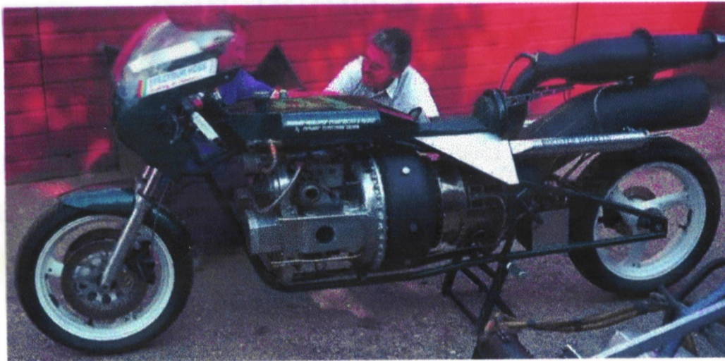
Motorcycle powered by a gas turbine – one of them is owned by Jay Leno
